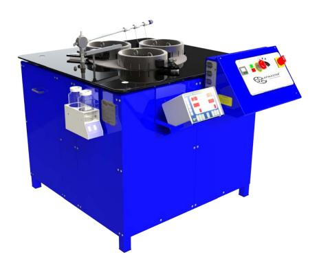
The Lapmaster Model 24 is the smallest floor standing lapping machine in the range and is ideal for engineering workshops, where flatness and finish are of prime importance. It is equipped with a 610mm diameter lap plate, faced with composite iron as standard.
